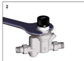
2- Using a 36mm wrench unscrew the upper part of the reducer
